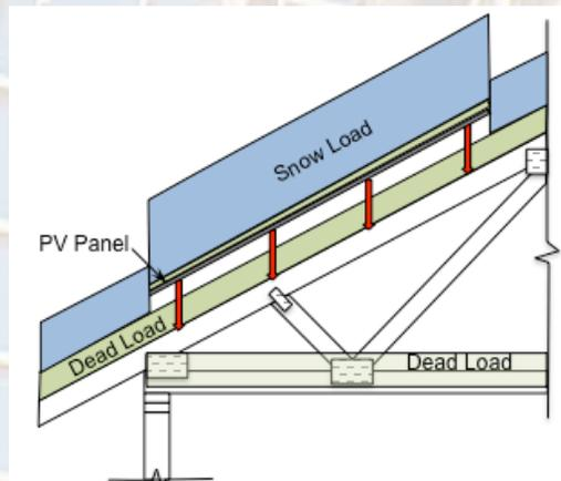
Fig. 2: Point Loads from PV Panel
